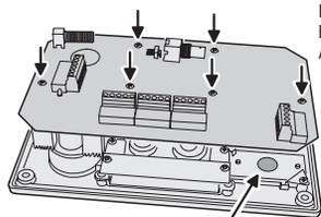
REMOVE THE SIX CIRCUIT BOARD RETAINING SCREWS AND FLIP THE CIRCUIT BOARD UP
